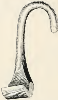
FIG. 37.—Curved chisel, used for the same purposes as Fig. 36. (One-half natural size.)
